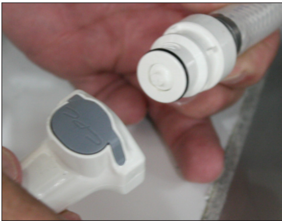
Fig. 21 Quick connect disengaged
