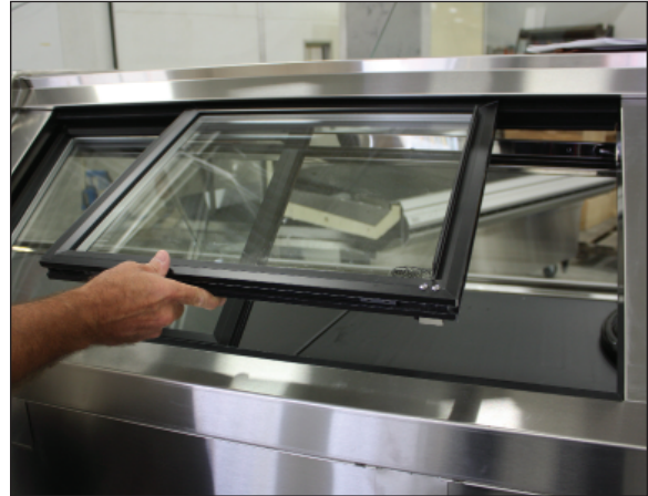
Fig. 18 Rear load door removal
